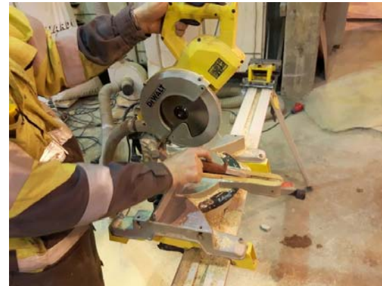
Cleaning of blade groove on circular saw.
