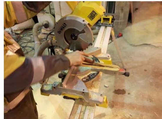
The employee stumbled causing the blade guard to open and the rotating blade hit his fingers.
