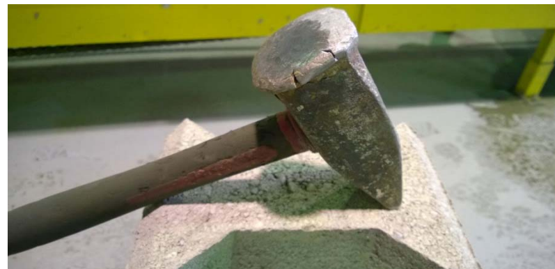
The sledgehammer from which the metal fragment came off.
