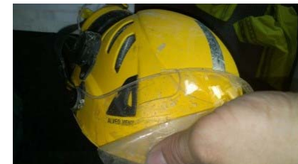
The protective visor on the driver's helmet was fractured and scratched.
