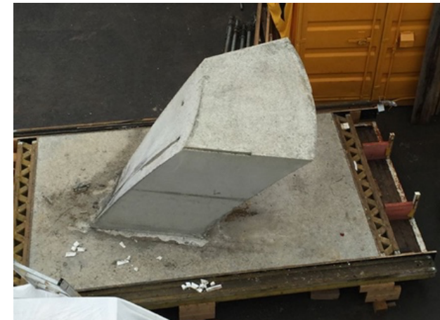
Photo: Voxeljet. Size of column: 1980 x 1082 x 289 mm 3
