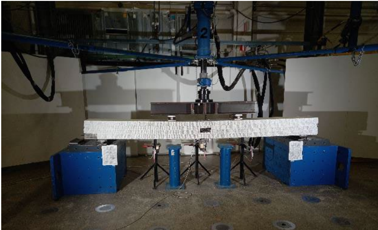
Bending test setup Min 10 Loading steps, each 3-5 minutes
