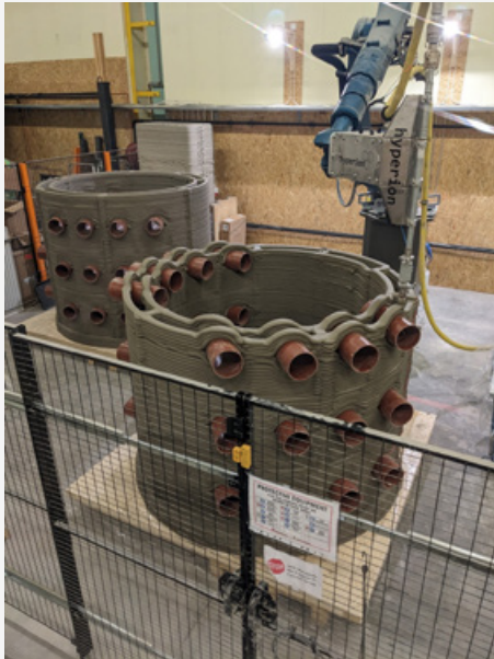
2 drawpits being manufactured by Hyperion's robotic arm.
